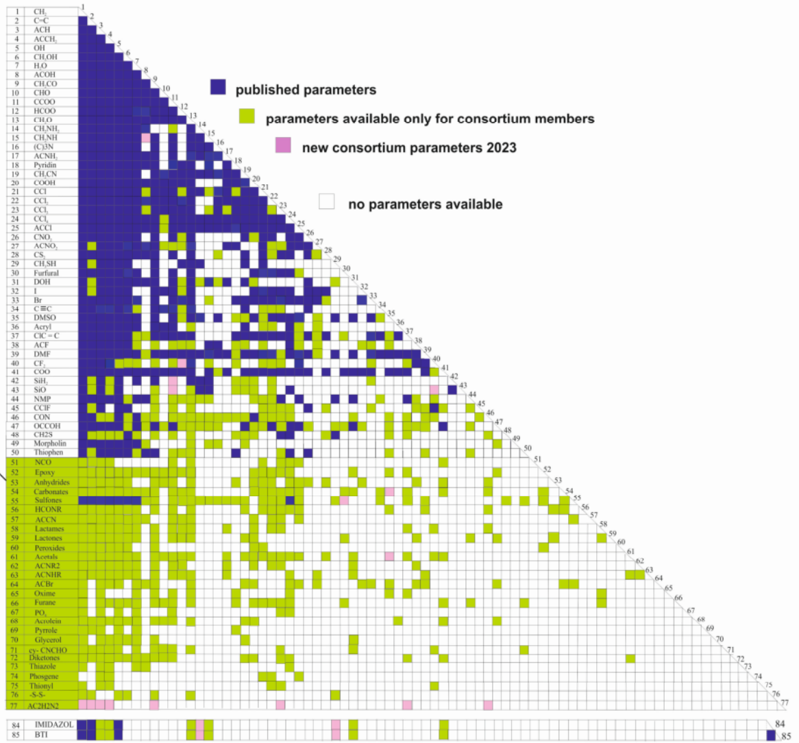
Fig. 4: Stage of development of the group interaction parameter matrix of original UNIFAC
